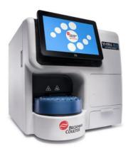
The Vi-CELL BLU automates the widely accepted trypan blue dye exclusion method for cell viability that has historically been performed with a light microscope, pipette, and a hemacytometer. This makes it perfect for large-to small-scale cell viability/counting applications in many fields including biopharma and academia.
